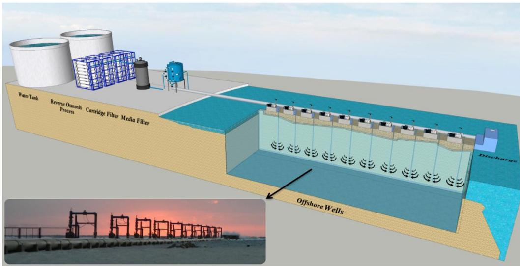
Figure 2. Offshore wells intake used to supply feed water to the studied SWRO facility
